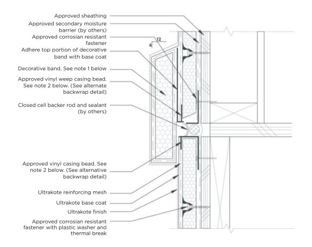
NOTE 1: Deocrative band shall be pre-wrapped with base coat and reinforcing mesh prior to installation. NOTE 2: Maintain 1/8" space between beveled insulation and weep casing bead. NOTE 3: At horizontal wall surfaces, including ledges, caps, sills, etc. a minimum slope of 6:12 is requires.
